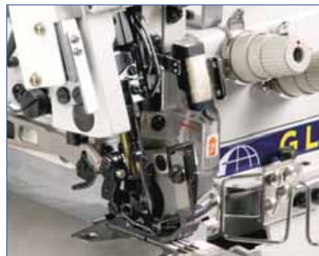
OV 614-408-TC • 2 needle 4 thread double chainstitch with Tape cutter
